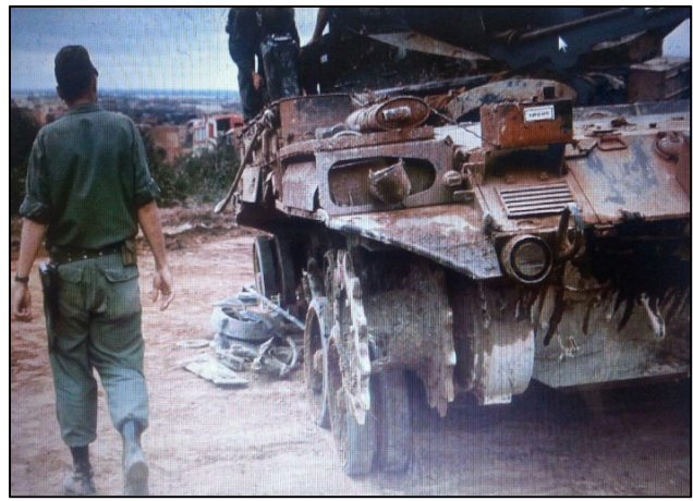
"A" Battery replacing blown track
