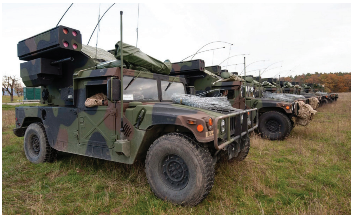
The U.S. Army brings back its Avenger surface-to-air missile systems mounted on a High Mobility Multipurpose Wheeled Vehicle, commonly known as the Humvee. (Photo: Georgios Moumoulidis: UAS Vision)
