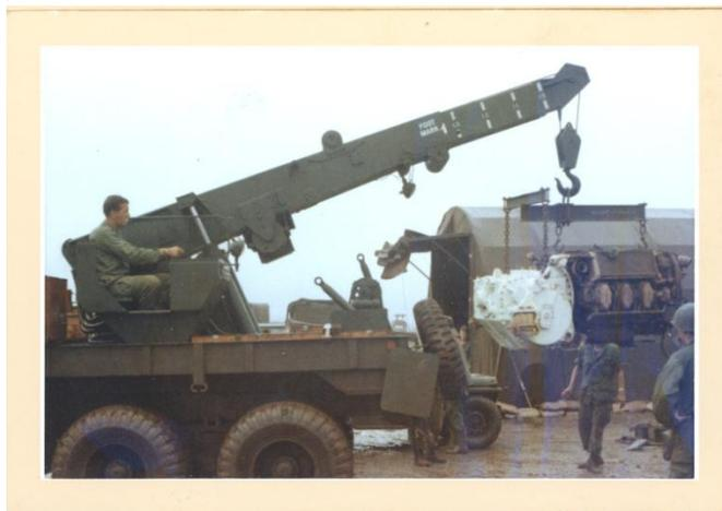
Late that afternoon we got a wrecker to pull the pack with a cracked piston. We had the new engine in at eleven thirty pm. It didn't take me long to get into bed. (*Note: I remember this. We were working under lights. On a forward fire base at night working under lights you feel like a great big target. You are just waiting for that mortar round.*)
