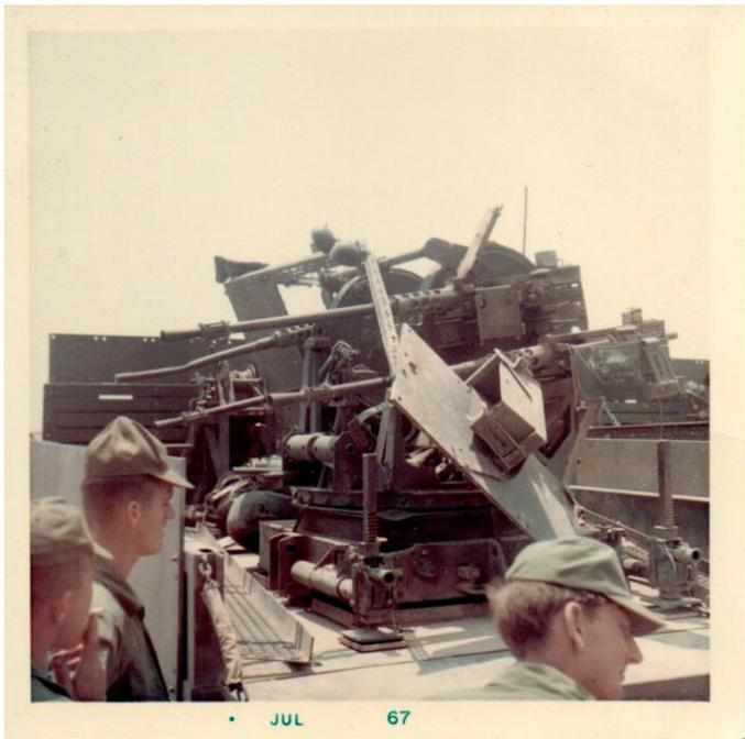
You can see that the gun side shielding “Bat-wings” are forced forward, indicating a force from behind. The UR barrel is melted.
