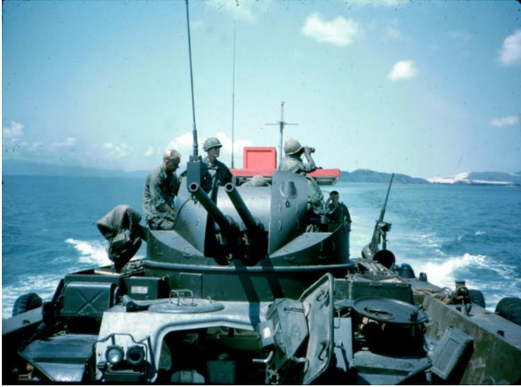
The use of a Landing Craft, Mechanical-8 (LCM) as a firing platform and transport for the twin 40mm gun, M-42 was tested during January 1968. The area of operation was in the Qui Nhon bay area.
